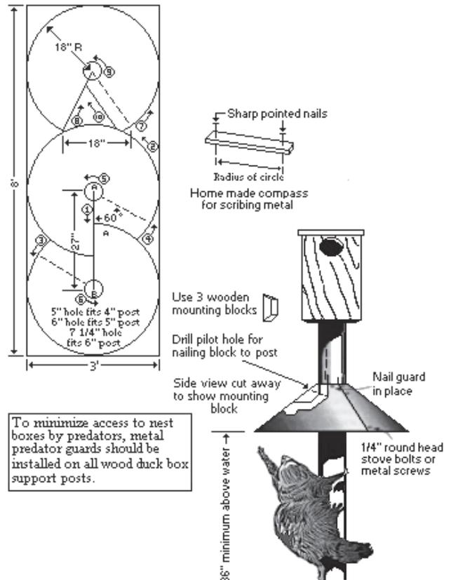
the guard, overlap the cut edge to the dotted line. To facilitate cutting, follow the sequence of numbers. Make circular cuts in counterclockwise direction. To make initial cut on line A-B, make a slot at A with a wood chisel, use tinsnips, and wear leather gloves.
