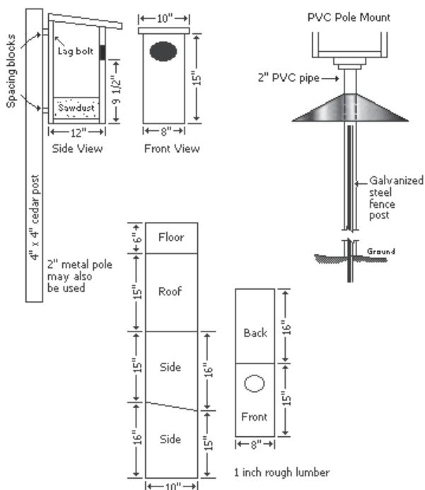
Figure 2 - Standard cone-shaped predator guard
